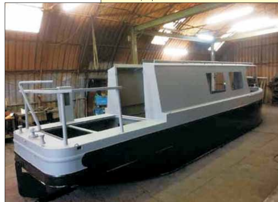
Bottom Left: Mike McHugh (in mask) examines the build in progress and anticipates being at the tiller! Above & Below: The two-tone finished shell ready for its fit-out and propulsion systems. The bow thruster port (above) will give the extra manoeuvrability required for this 32' craft.
