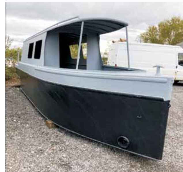
Bottom Left: Mike McHugh (in mask) examines the build in progress and anticipates being at the tiller! Above & Below: The two-tone finished shell ready for its fit-out and propulsion systems. The bow thruster port (above) will give the extra manoeuvrability required for this 32' craft.
