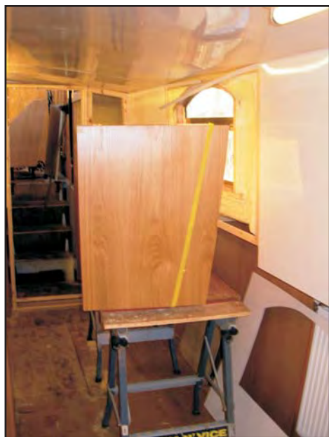
The yellow tape shows how much wasted space there would be if I accepted the 'joiners' refusal to use the boat side as the unit back.
