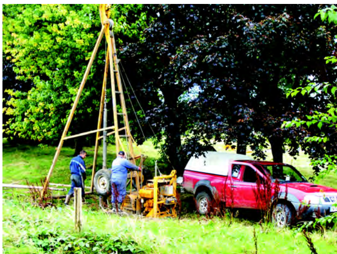
Taking core samples at Droylsden with a portable drilling rig.
